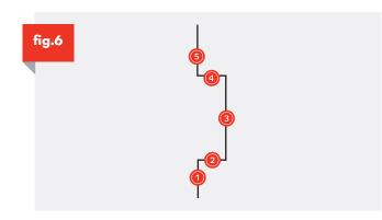
**2.1.** Measure from the flat face of skirting board 1 to the external corner of the wall. Cut the skirting board using square cuts. Fit a scribed internal corner moulding to the left hand end and check for fit. If satisfied fix in position with adhesive. See **Fig 5**
