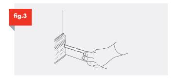
**1.4.** Apply contact adhesive to the scribed internal corner moulding (available from your local Eurocell Building Plastics branch as part of the corner trim kit) and push onto the left hand end of the cut skirting board. Position the skirting board to check for length and trim if necessary. Once satisfied repeat stage 2. See **Fig 4**
