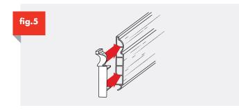
**2.2.** Measure length 4 from the inside corner of the room to the external corner of the room. Cut to length using square cuts. If satisfied with fit fix to wall using adhesive.
