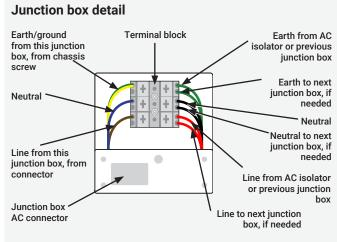
**f.** Gently arrange all the wires and connectors inside the junction box and replace the cover. Tighten the cover screw using a Phillips screw driver.
