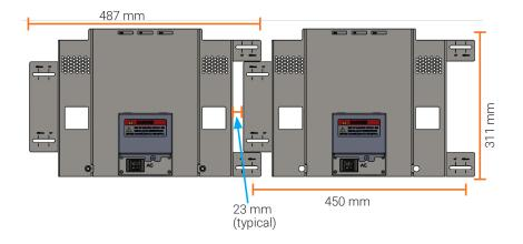
BWM-600MM-A allows 600 mm battery-to-battery spacing:
