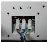
Fig. 8 AC terminals under AC terminals cover
