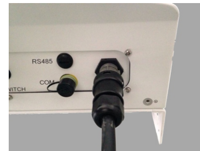
▲ Figure 4.14 Connect the Terminal Connector to Solis-15K
