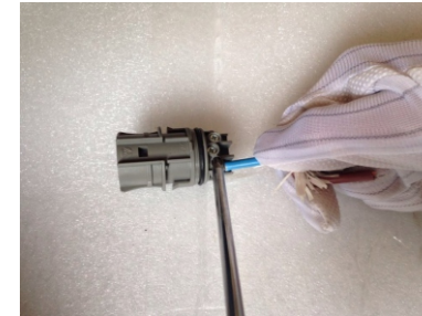
▲ Figure 4.12 Connect Wires to the Grid Terminal
