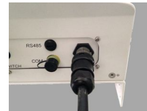
▲ Figure 4.14 Connect the Terminal Connector to Solis-4.6K-2G
