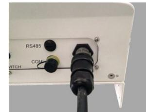
▲ Figure 4.14 Connect the Terminal Connector to Solis-5K-2G
