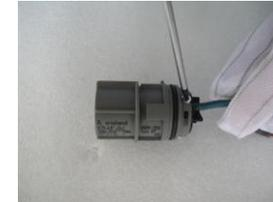
▲ Figure 4.12 Connect Wires to the Grid Terminal
