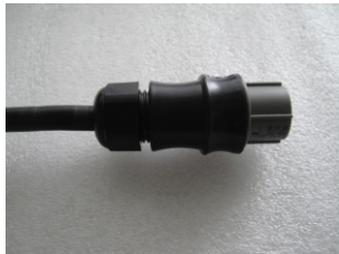
▲ Figure 4.15 Tight Up the Cap on the Terminal
