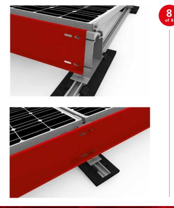
Use two standard module middle clamps each between two modules which are also fastened with bolts with serrated under head M8 screws in the M K2 slot nuts.
