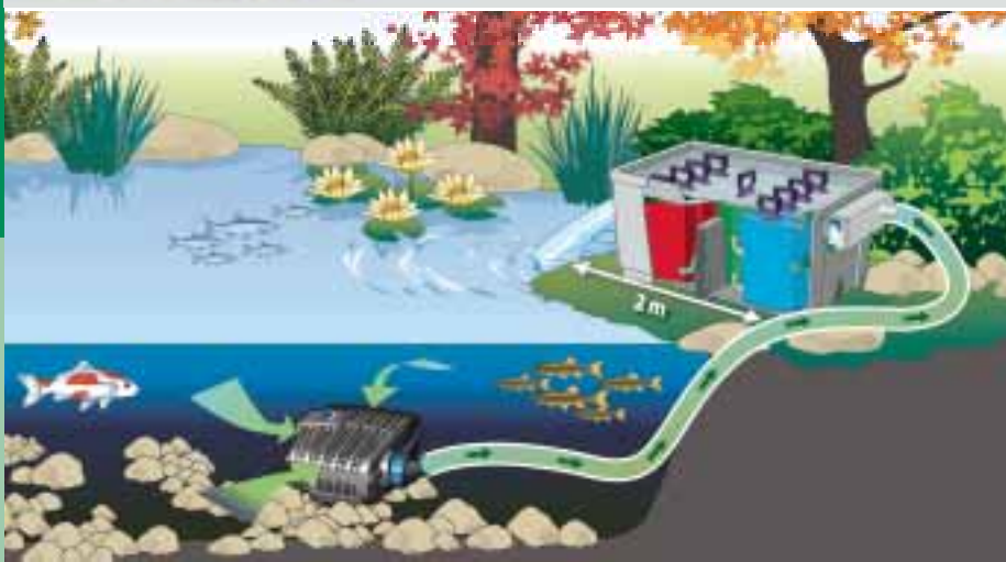
Schematic diagram: BioSmart 30000 in combination with filter and watercourse pump AquaMax Eco Classic
