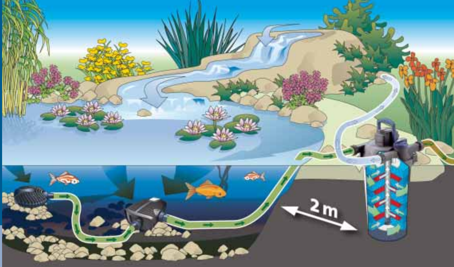
Schematic diagram: Filter and watercourse pump AquaMax Eco (PRO) in combination with an OASE pressure filter FiltoClear (PRO)
