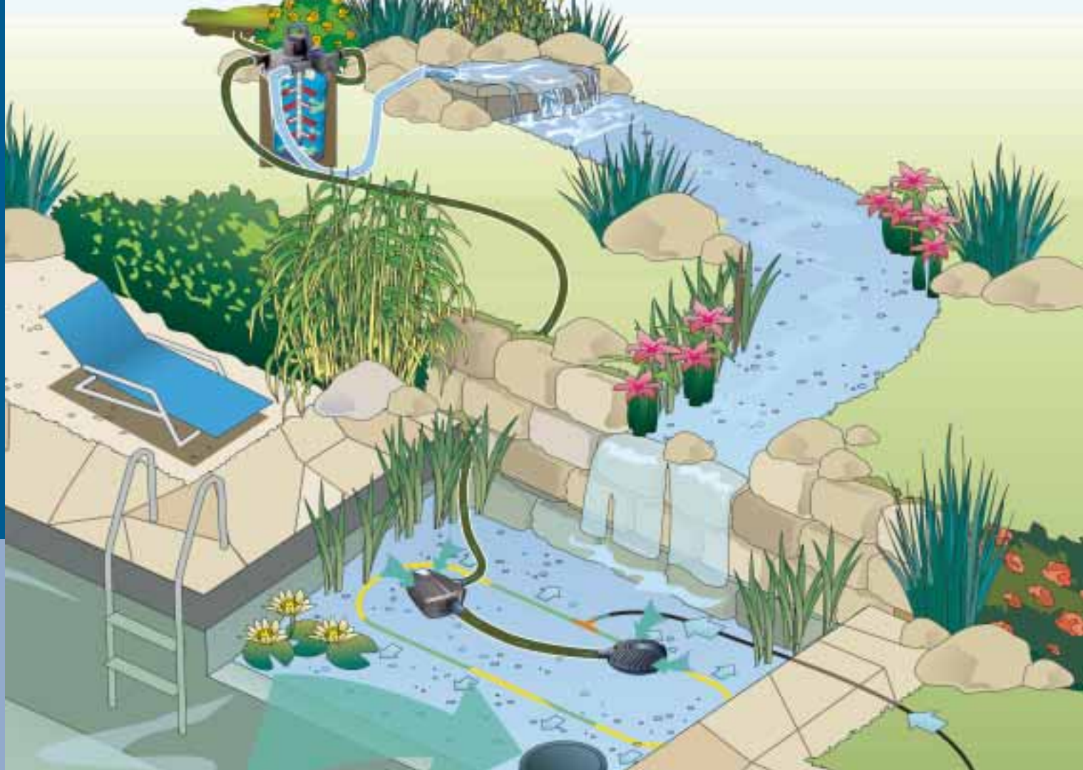
Schematic diagram: Filter and watercourse pump AquaMax Eco Premium 12 V (PRO) used in the swim pond in combination with an OASE pressure filter FiltroClear (PRO)
