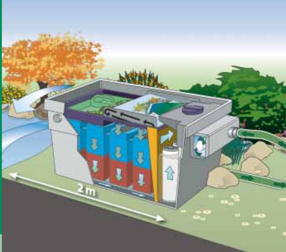
Schematic diagram: UVC in combination with OASE BioTec ScreenMatic
