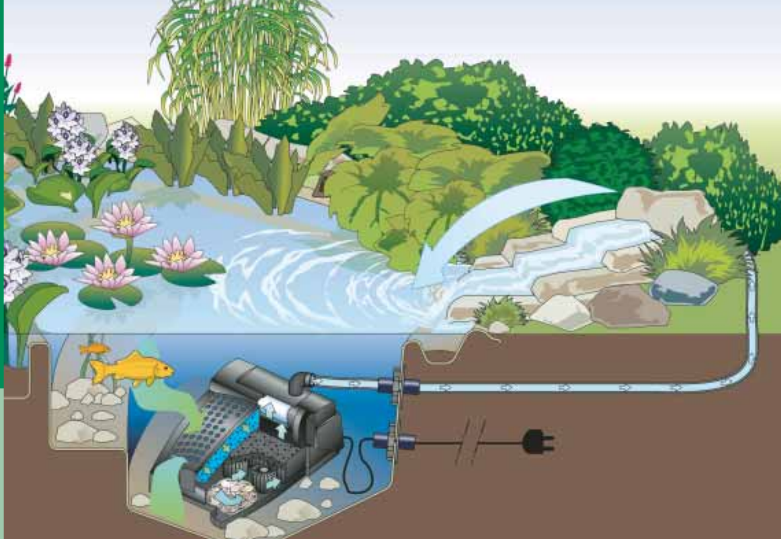
Schematic representation: Underwater filter Filtral UVC (GB-Version) inserted in a pond
