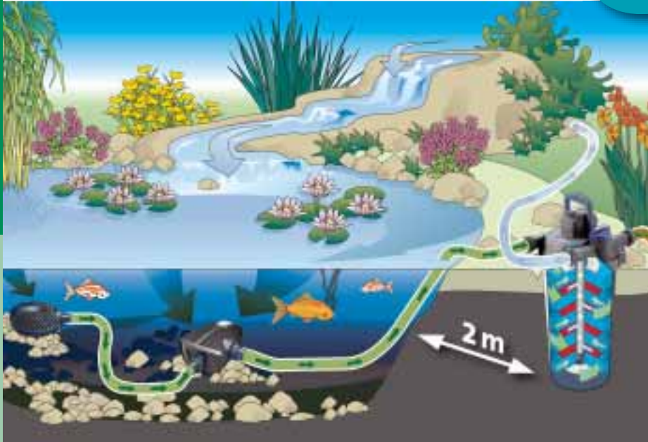
Schematic diagram: Pressure filter FiltoClear in combination with filter and watercourse pump
