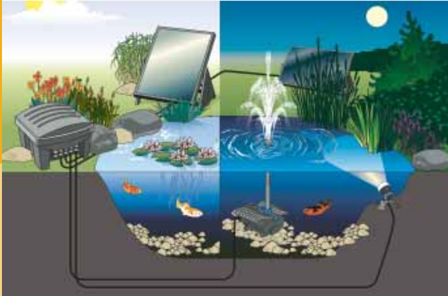
Schematic diagram: Interaction of the different solar components
