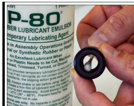
Fig. 2b | Apply seal lubricant to inside of rotary portion of the seal with cotton swab.
