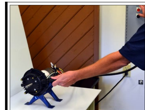
Fig. 12b | Bump start the motor to verify wiring and operation.
