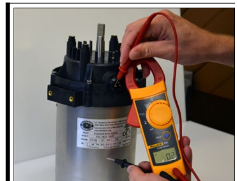
Fig. 1c | Check for continuity between S/S housing and ground pin on bulkhead to confirm that S/S housing and ground clip are touching.
