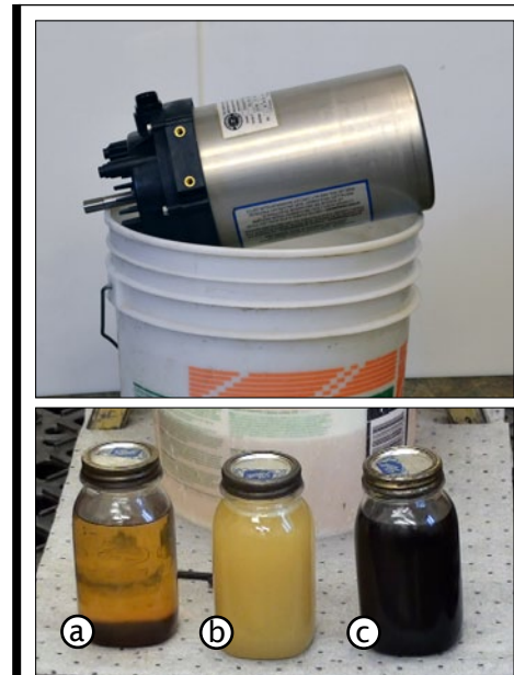
Fig. 2c | [Top] Remove oil plugs and drain oil, note condition of oil. [Bottom] Condition of oil: (a) Clean Oil (b) Milky Oil (c) Dark Oil
