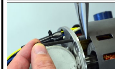
Fig. 7a | Partial removal of endbell may be required to replace protective sleeves on motor bolts.
