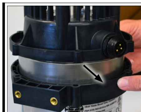
Fig. 15b | Make sure two flat areas of the Housing Ring align with the bulkhead or hardwire cable assembly & oil plugs.
