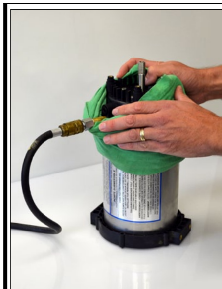
Fig. 2a | When removing motor base plate with air pressure, wrap a rag around the assembly to catch excess oil.
