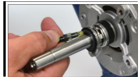
Fig. 4b | Apply one drop of 3-in-1 oil onto face of rotary portion of the seal.
