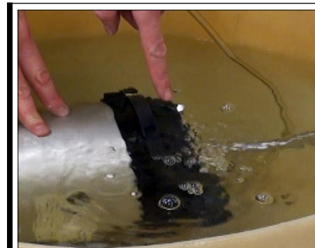
Fig. 16b | Water dunk tank works well for testing leakage, you can also use a soapy water solution.
