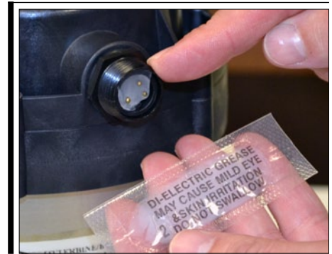
Fig. 17b | Place dielectric compound or silicone grease in the bulkhead connector to prevent water penetration which will lead to nuisance tripping.
