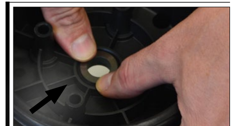
Fig. 5b | Apply seal lubricant to outside surface of rubber seal seat cup and insert it into counter bore of MBP with seal seat facing up, press firmly.
