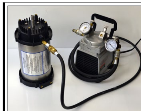
Fig. 14b | Draw motor base plate assembly into S/S housing using 20 in. Hg of Vacuum.
