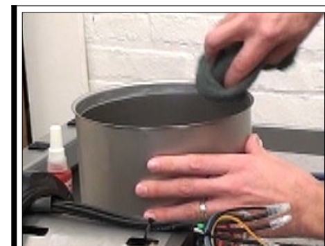
Fig. 13b | Wipe seal lubricant around the top of the S/S housing to help with seating the motor/motor base plate assembly.
