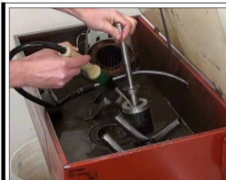
Fig. 4a | If water was present in oil, you might be able to reuse motor. Separate motor rotor and stator and wash both in mineral spirits; allow to dry overnight before retesting.
